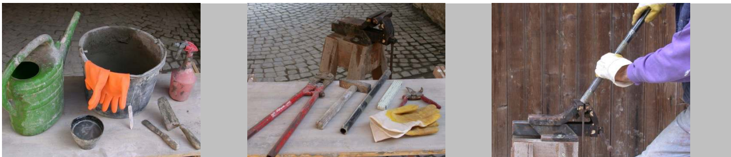
The most important tools for working in build-up technique at a glance: Watering can, plaster cup, construction bucket, rubber gloves, modelling tool, spatula, trowel, spray bottle, vice, bolt cutter, hammer, steel pipe, folding rule, rose shears, work gloves. The vice and the piece of pipe help to bend the rebar. With it, even short ends can still be grabbed and bent at quite a sharp angle..
