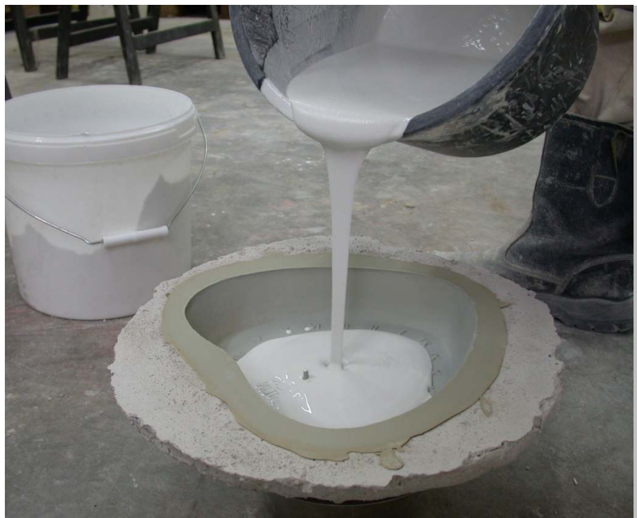
A self-compacting concrete runs into the mould like honey. If you pour it in a thin stream, you can avoid unwanted air pockets. It must not be vibrated, because the retained superplasticiser could cause it to segregate.
