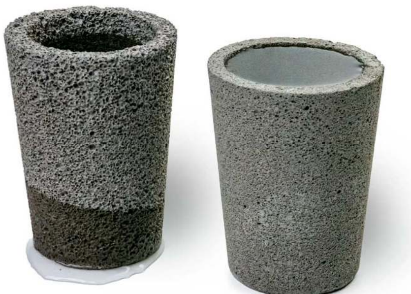
Although it is extremely porous, foamed concrete can also be made waterproof by adding hydrophobic agent. The right cup was sealed with PREN.
