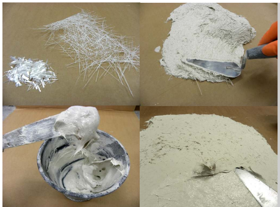
In the ultralight concrete technique, the special cement WUTZ is mixed with two types of AR glass fibres (picture above left): fine short fibres for the top layer (left in picture) and coarse glass fibre mat for the substrate (right in picture). The substrate mortar is applied only 1-2 mm thick per layer (picture above right). The fine top coat mortar (picture below left) is finally applied even thinner to smooth out only the unevenness (picture below right).
